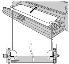
8 While restraining the center of the roll media, turn the roll holder to take up any buckle in the media, pull the roll release lever toward you, then lock the paper guide.
